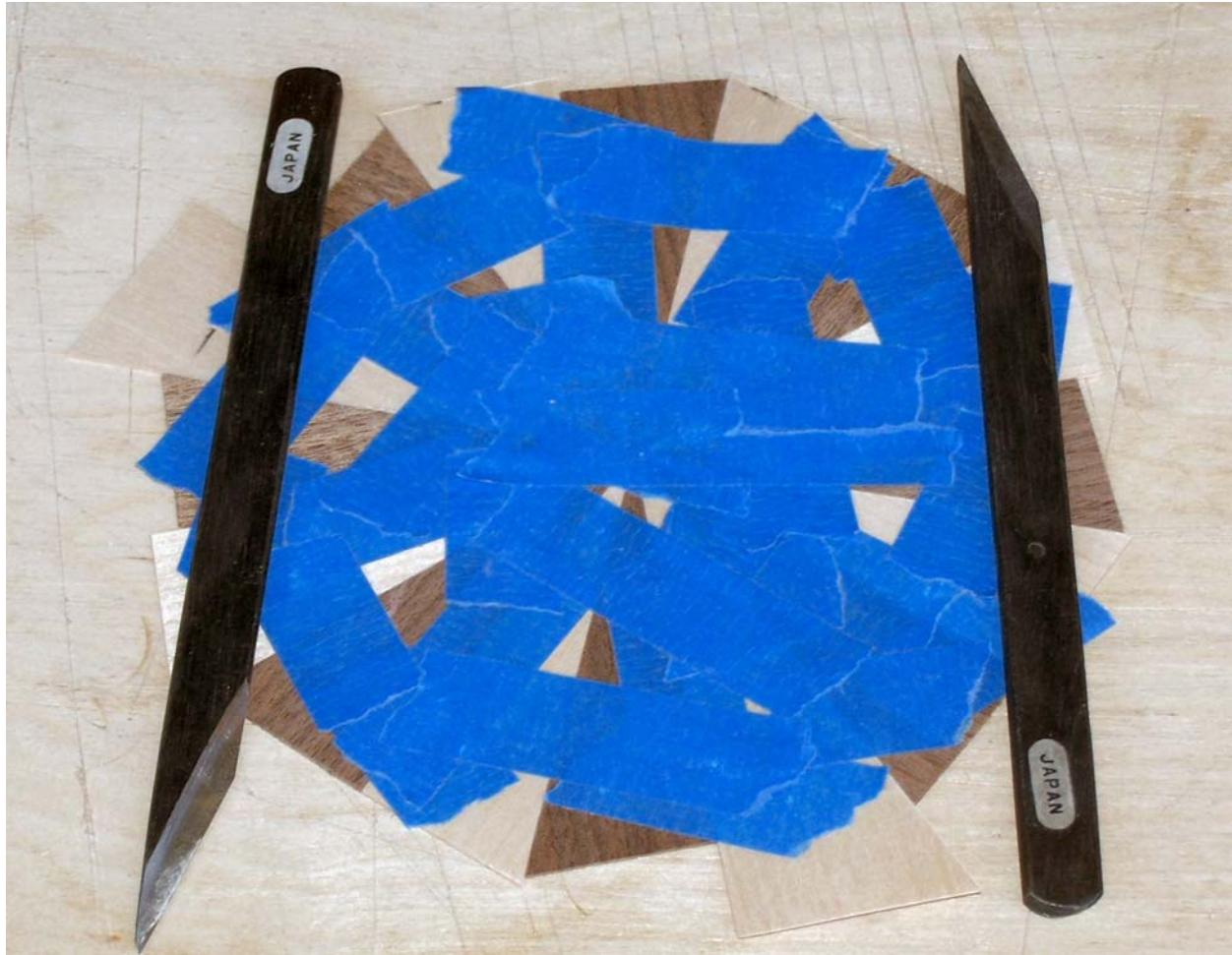
Now, turn it over so that the show face is up and begin putting veneer tape on the seams. Note that we don't want to have more than four layers of veneer tape at any point so you don't want to just run veneer tape across the face of the rose, over and over.
