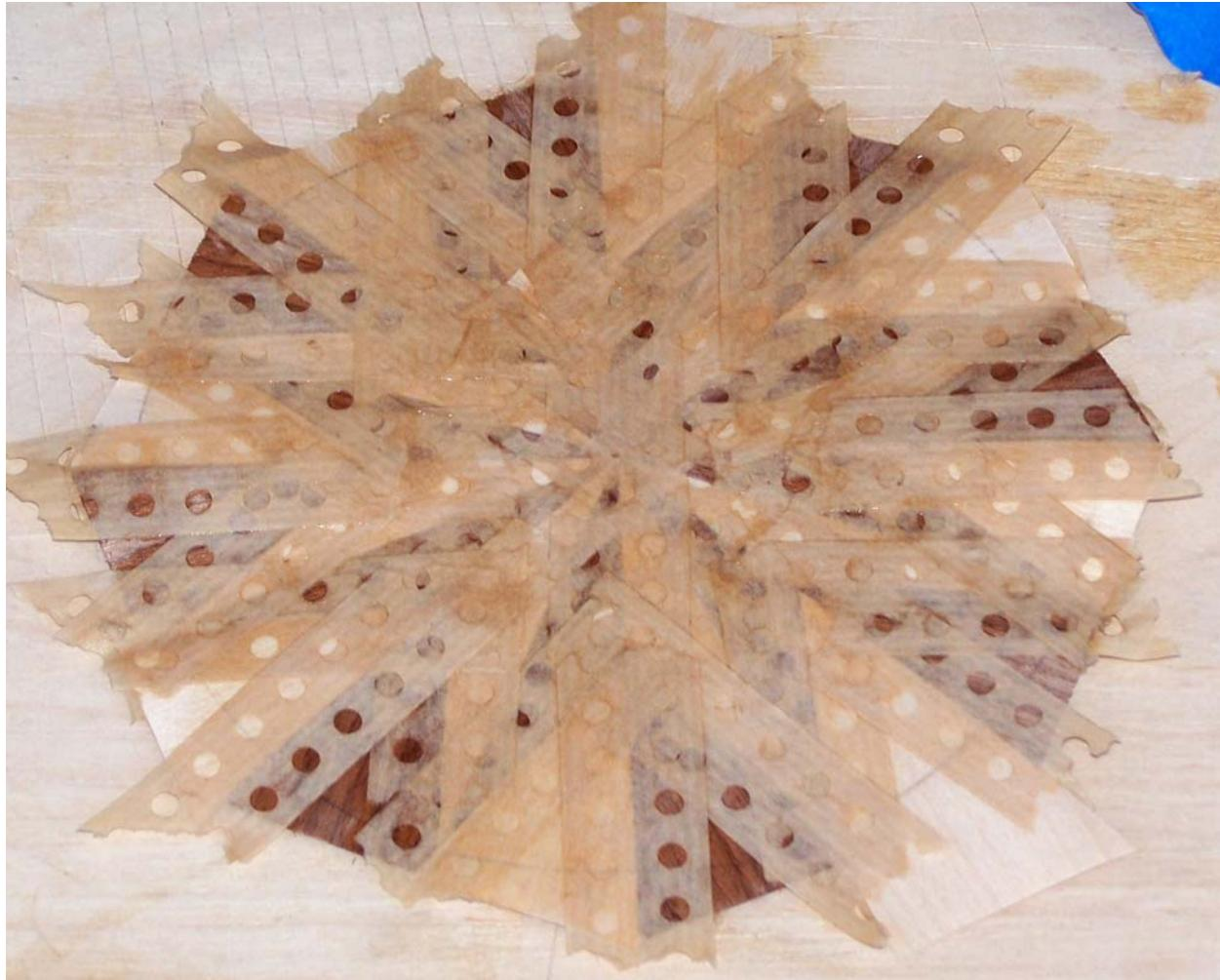
Set the piece aside and let the veneer tape dry well. Our next step is to turn the piece over and remove all the blue tape and the veneer tape from the glue face. The veneer tape on the show face must be dry and holding the pieces well or we'll have a mess on our hands.
