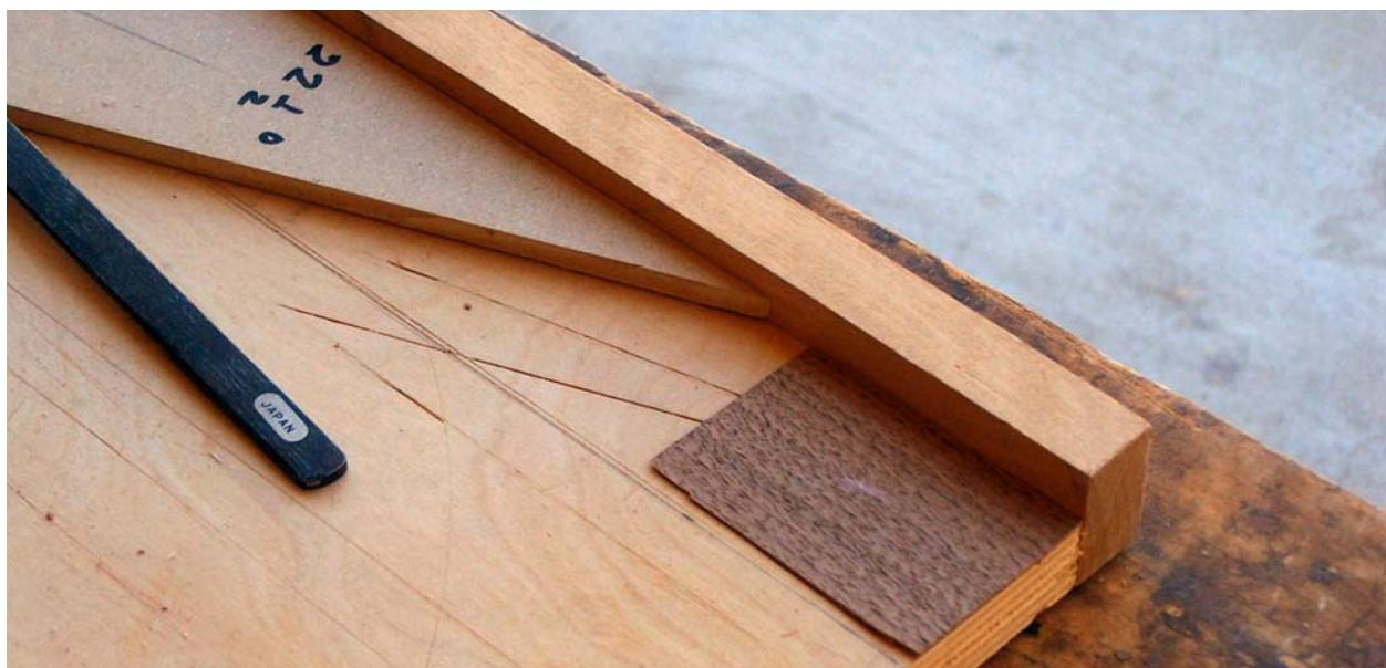
And then put the template over the piece of veneer to cut it. I cut it with the Japanese marking knife.
