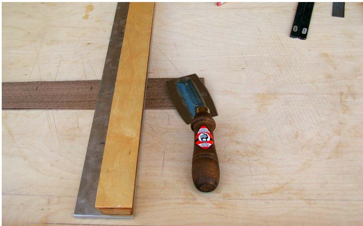
I used my veneer saw to cut the pieces to length. Ideally, you should mark the veneer so that you can maintain its orientation. That is, you want the same side up and the same direction pointing out from the rose. While this is good practice, if the wood is pretty consistent and
