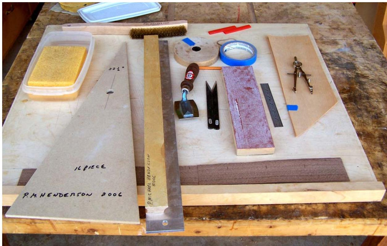
Starting from the left, we have a sponge sitting in a container of water. This is used to wet the veneer tape. Next, is the template for cutting the pieces of veneer for the compass rose. This template is for 16 pieces to make up a disk. You can make your own template but describing how to make one, and verify its accuracy, is beyond the scope of this article. Above the template is a brass brush which is used to brush the veneer tape after it's applied to get it to lay smooth.
