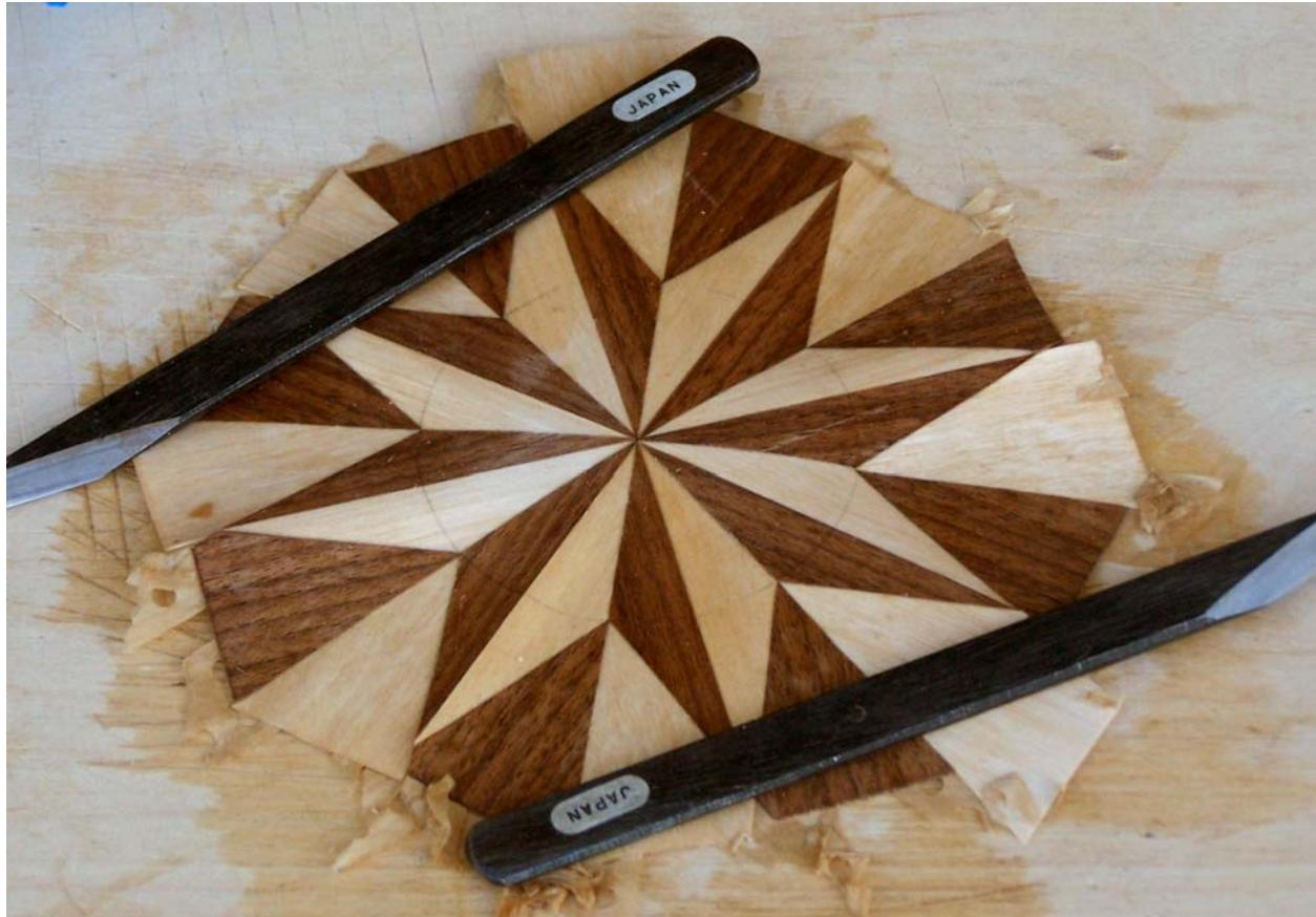
Since we put water on the piece to remove the veneer tape, we need to set it aside and let all the water dry before taking the next step.
