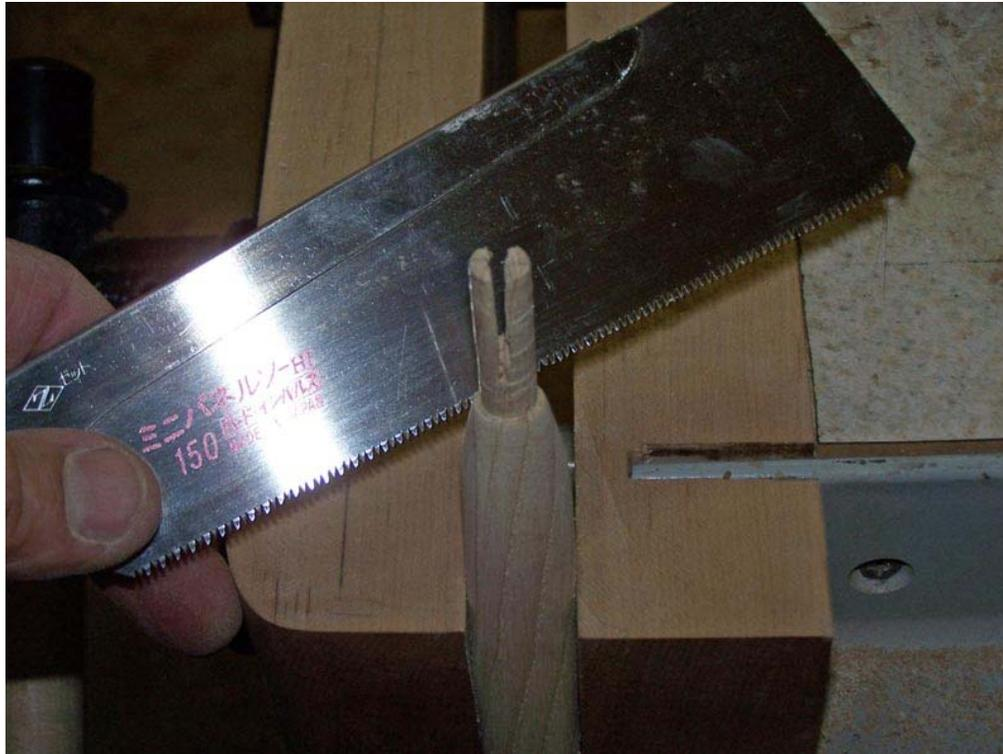
Next, I need to cut the wedge. I took a piece of scrap and cut it to 3/8" wide. Then I mount it in my vise and use my saw to cut a wedge shaped piece off of it. While not shown, I cut the end of the wedge off so that it will go down into the slot.
