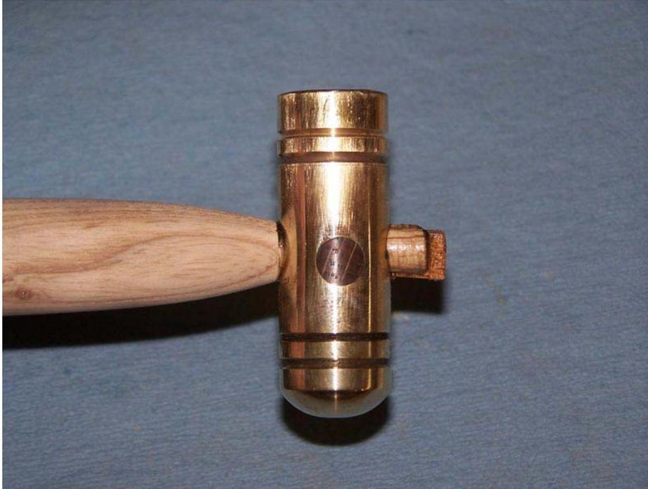
When the epoxy is well set, I cut off the excess on the band saw, then trim the handle flush with the head with a chisel.
