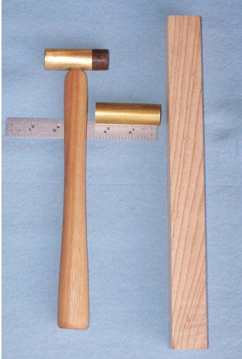
I'll begin by creating the dome on the brass stock. To do that, I mount the brass rod in my lathe using a chuck.
